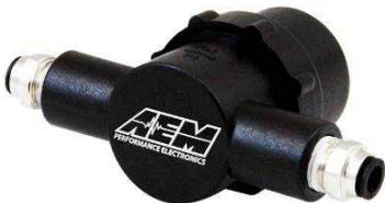
Inline filter that uses a micronic mesh screen to filter out particles as small as 40 microns. Allows a cleaner flow of water/methanol into the injection pump, lines, and nozzles increasing overall system longevity. Injection filter is **HIGHLY RECOMMENDED** when using the AEM water/methanol injection flow gauge.
