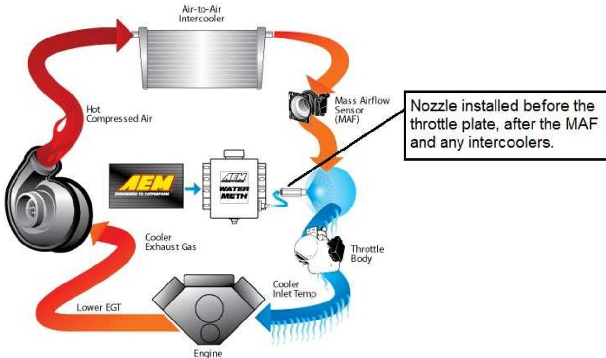
In most instances, the air charge piping can be drilled and tapped for 1/8" NPT to directly mount the nozzle. If using thin walled tubing it's suggested that a bung be welded to the piping. Mounting hole should be tapped deep enough to allow the end of the nozzle to be nearly flush with the interior of the intake once the nozzle is fully installed.
