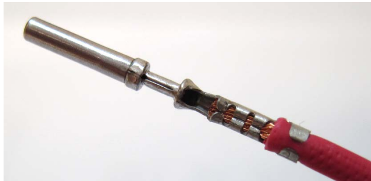
Image shows a properly crimped terminal. Top View.
