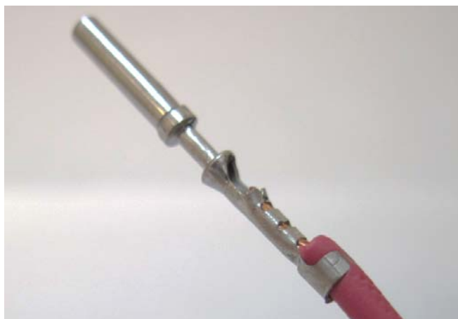
Side View. After crimping, be sure to do a pull test to make sure the terminal is properly installed.
